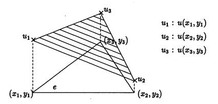
Let  $\hat{u}(x,y)$  be a piecewise linear function which approximates u(x,y) on a finite element e, then we can write
